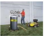
Sandblaster: For dust-free stripping of paint from walls, barnacles from ships, etc.
